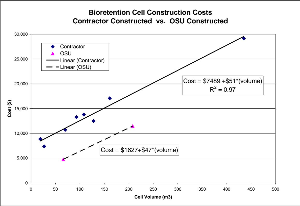
Figure 2. Comparison of Bioretention Cell costs; contractor versus OSU constructed cells.
