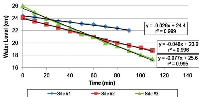
**Fig. 4.** Typical graph of double-ring infiltrometer inner ring depths versus time. Linear regression lines were applied to the data to determine the surface infiltration rate. Data presented are specific to the dry, scoop test plot at the Nashville site.
