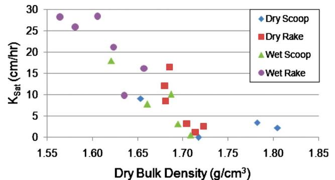
**Fig. 5.** Saturated hydraulic conductivity versus dry bulk density for the Nashville site.
